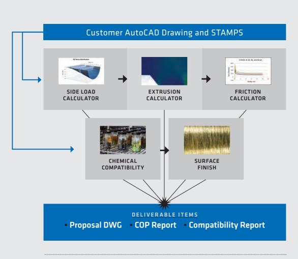
This graphic shows the Cylinder Optimization Process through its sequential steps. The information it produces uncovers ideal parameters to design and position guide bands, sealing systems and other opportunities to optimize a cylinder's performance.
