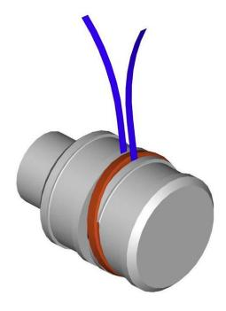
4. After the piston seal is completely installed into the seal groove, let go of one end of the strap and pull the strap from underneath the seal ring. Installation is complete.
