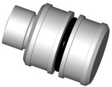
2. Using a nylon strap, lasso the seal ring, and by hand, engage the opposite end of the seal ring onto the piston. Holding the nylon strap, modestly pull the seal ring over the top of the piston, adjusting the nylon strap's position as necessary to work the seal ring over and onto the piston. Take care as to not over-stretch the seal ring and cause permanent deformation.
