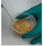
8. Apply adhesive with brush to seal and both sides of dowel pins. Insert dowel pins into either half of seal.
