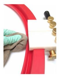
11. Loosen and remove red clamp screws and upper clamps. Remove seal from fixture.
